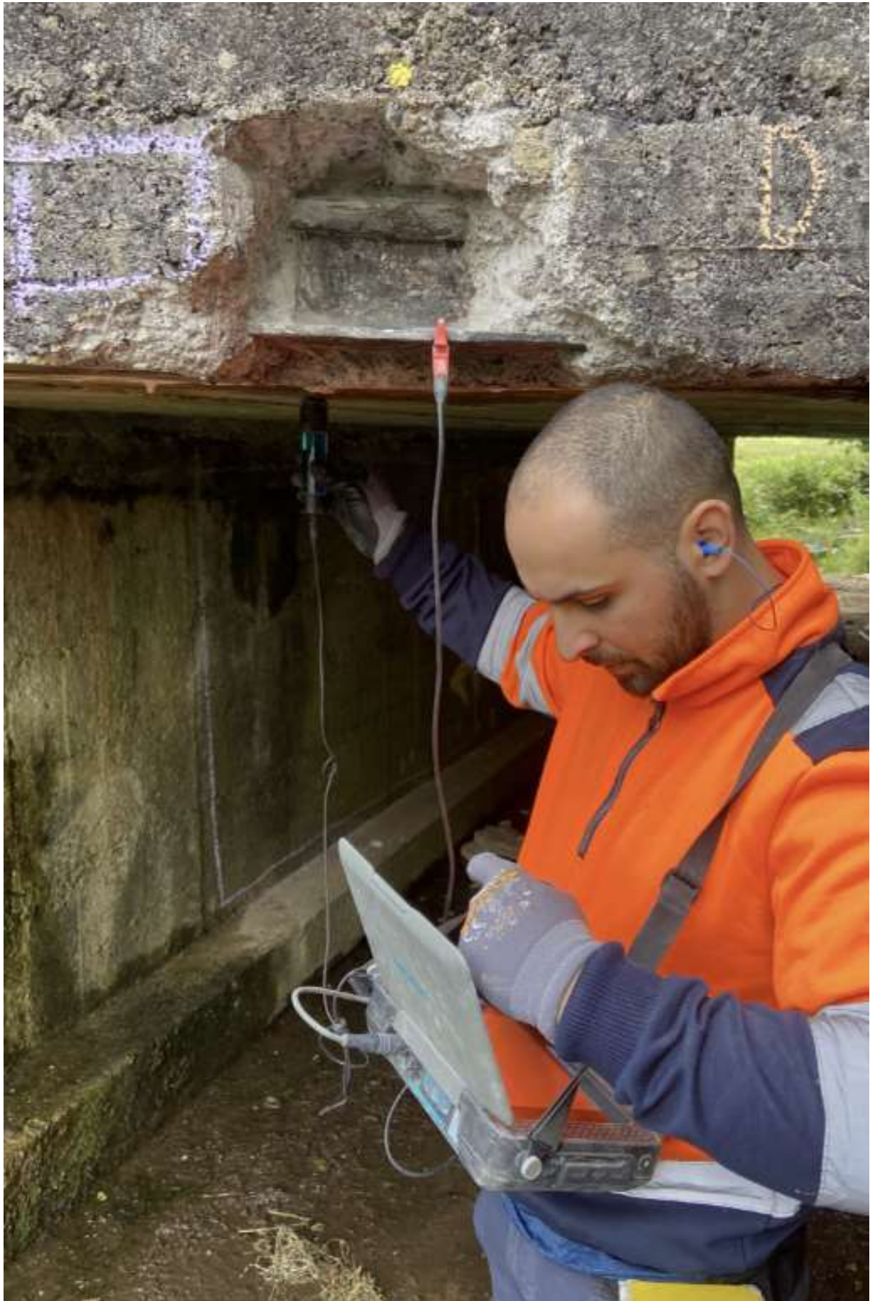
Figure 22: Half cell potential testing
