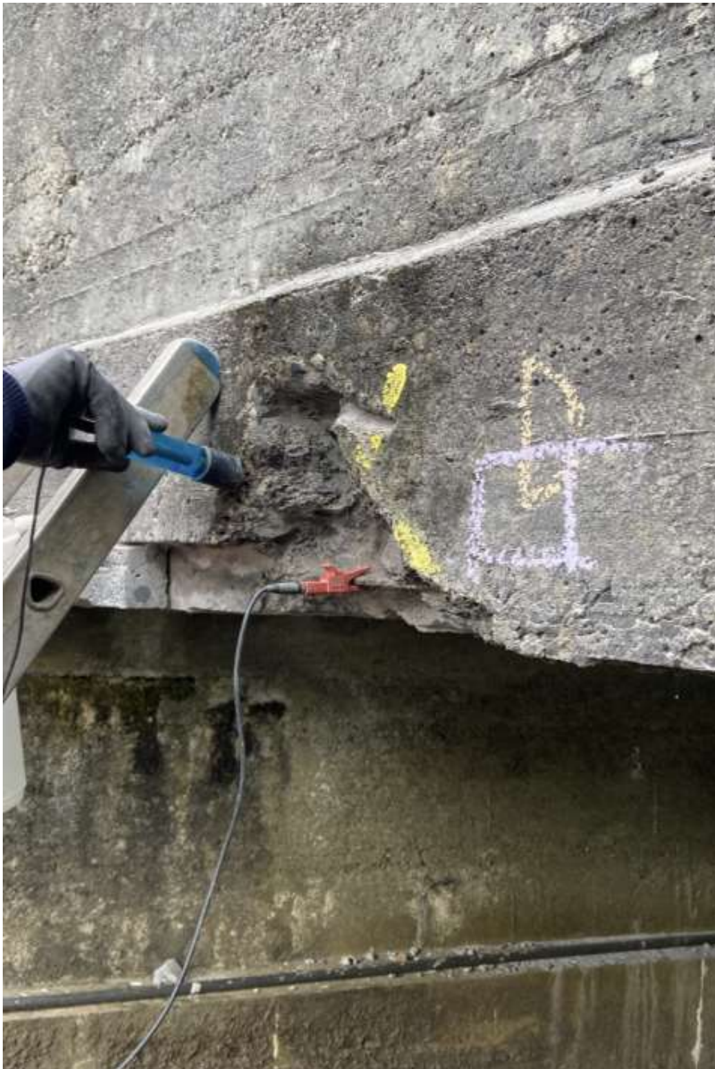
Figure 32: Half cell potential testing of TP04
