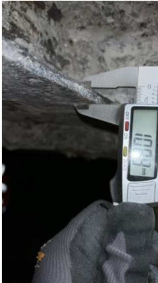
Area 3 - Bottom flange 124mm width
