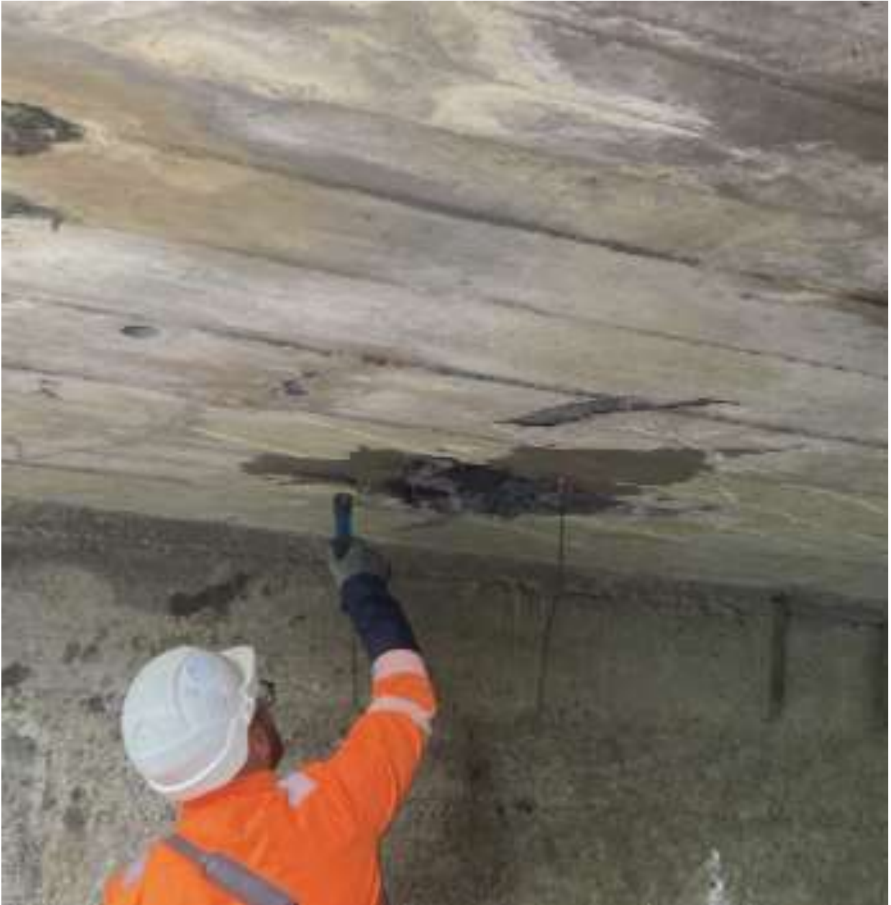
Figure 36: Half cell potential testing
