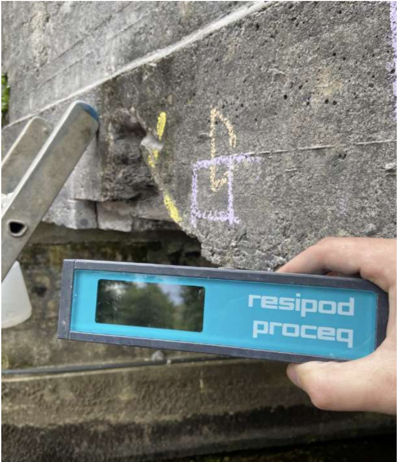
Figure 33: Resistivity testing of TP04
