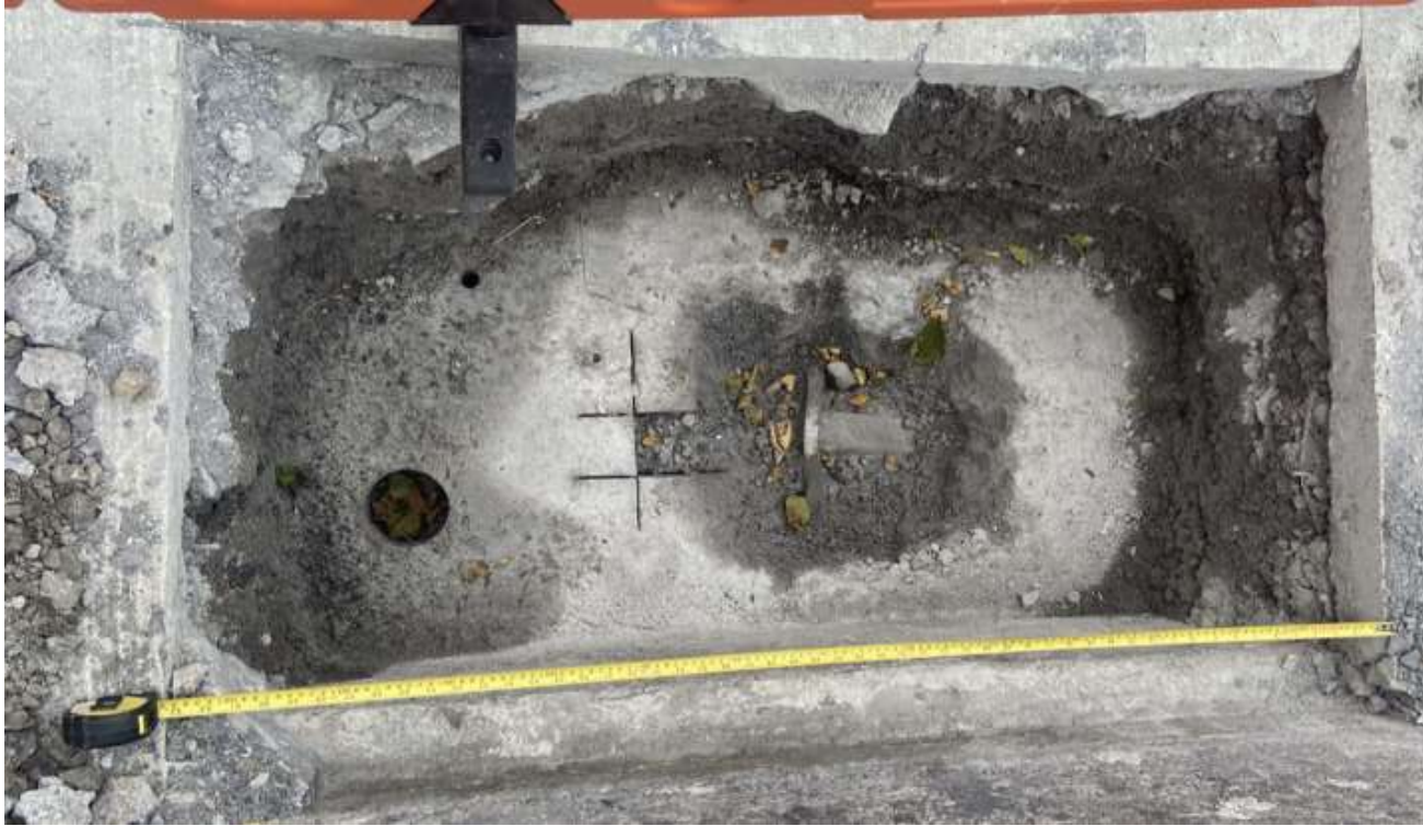
Figure 12: Test area 1 containing pilot hole, core sample hole and breakout.
